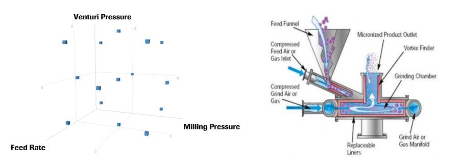
Full Factorial (+) Design studied effect of Feed Rate, Milling Pressure and Venturi Pressure on amorphous content.
