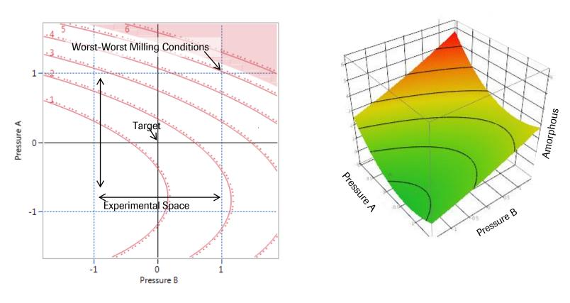
Jet milling of API within the proven acceptable ranges for the process parameters will produce Drug Substance with an amorphous content that is considered acceptable (typically ≤5%).
